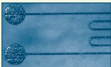
Laser micro-machined serpentine channels and bond pad filled with Parmod VLT copper ink (channels 12- \mu m wide by 9- \mu m deep in 3-mil thick Kapton® film).
